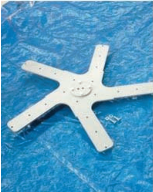
AFTER DISASSEMBLED BLADE SUPPORT, DISASSEMBLY HUB
